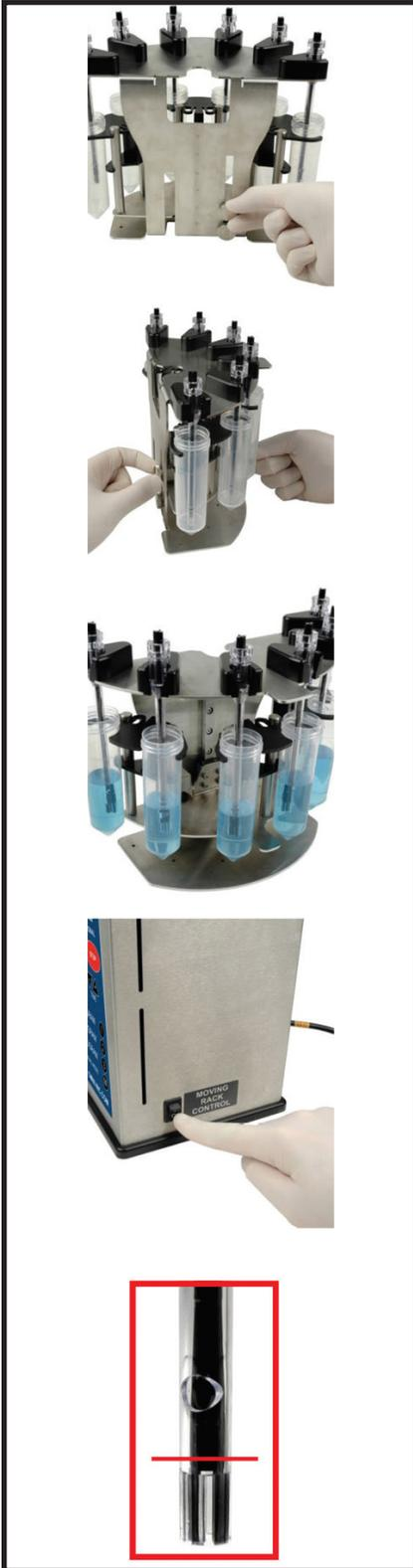
1. Load the tube holders, sample tubes, and disposable/stainless steel probes by following the steps (50 mL tubes shown).
