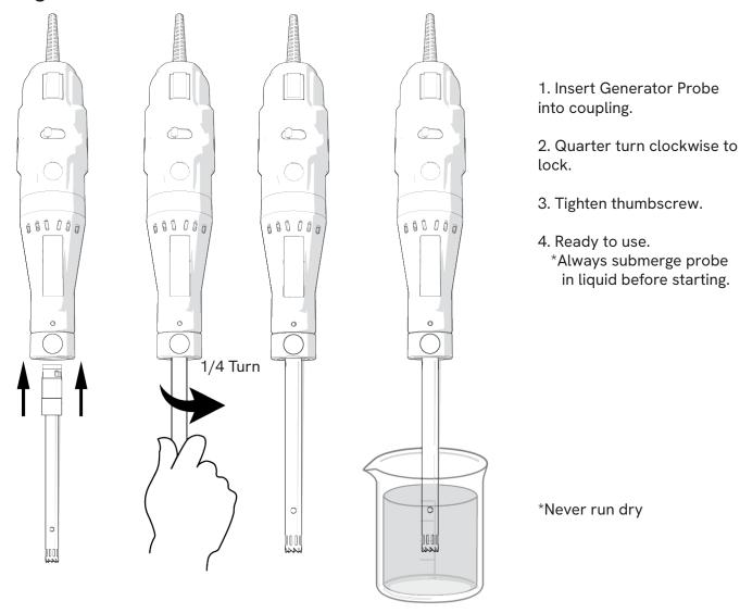
WARNING: The blue protective cap must be removed from the end of the generator probe before operating.
