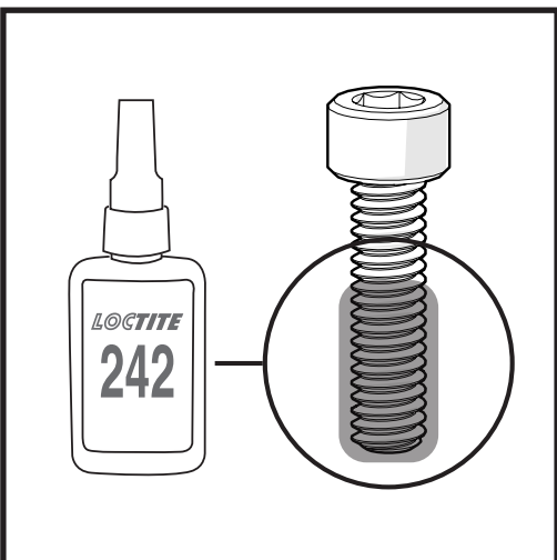
5. Apply Loctite adhesive to 8-32 x .75 screws before installing.
