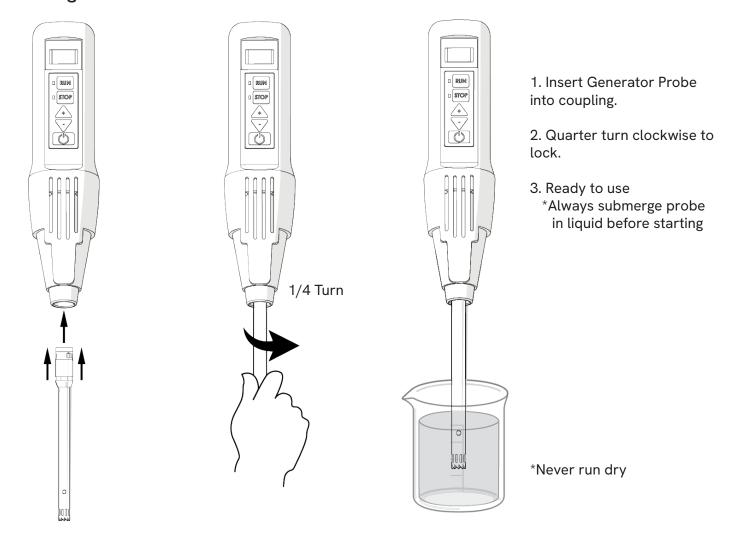
WARNING: The blue protective cap must be removed from the end of the generator probe before operating.
